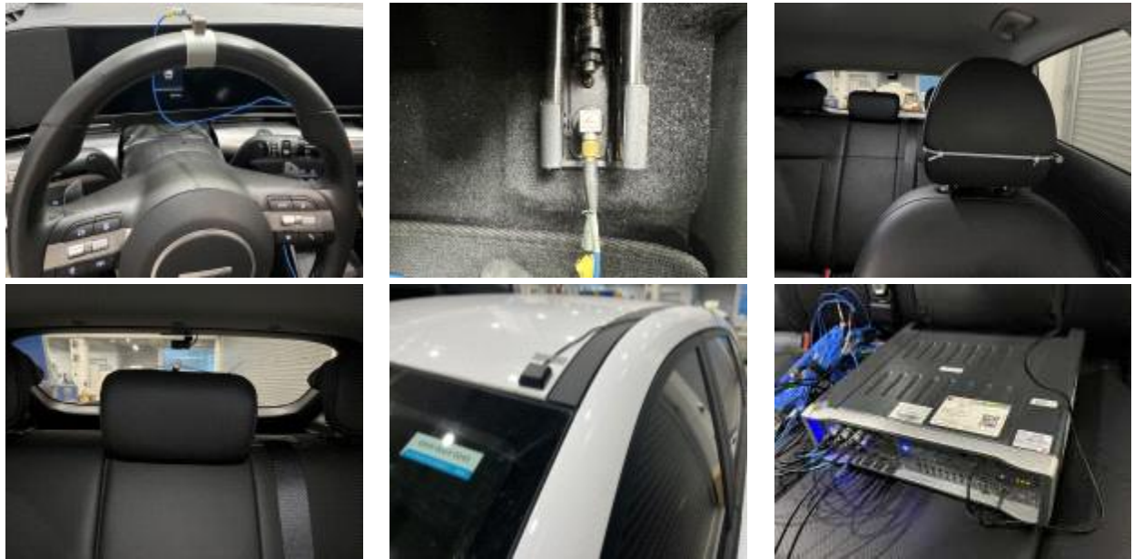
Fig. 2 Experimental setup for NVH data acquisition: (a) steering wheel accelerometer, (b) driver's seat floor accelerometer, (c) front-seat microphone, (d) rear-seat microphone, (e) roof-mounted GPS sensor, and (f) NVH data acquisition system.
